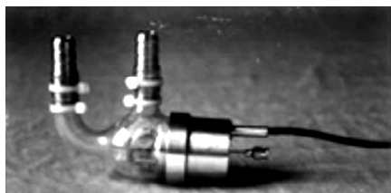
Figure 1. The implantable and pulsatile impeller pump for long-term circulation support.
